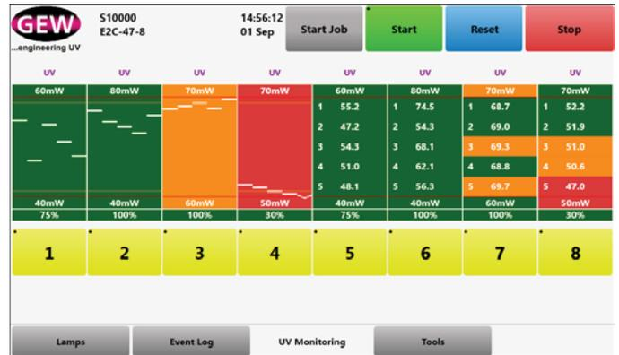
UV intensities for each lamp can be displayed in graphical or tabular form. Traffic light colouring warns when a lamp is approaching or exceeding set points.
